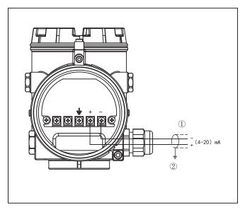
Electronics and terminal compartment, double chamber housing
